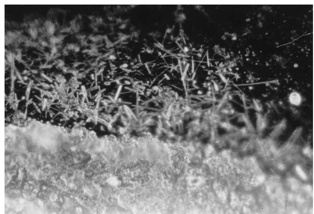
Figure 12 Whisker formation at the top surface of the glass layer.
